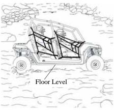
**WARNING!** The large tires on your vehicle may cause the vehicle to float in deep or fast-flowing water, which could result in loss of traction, loss of control, overturn or accident.
